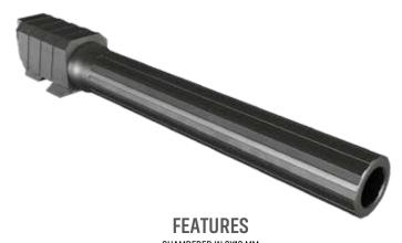
**CHAMBERED IN 9X19 MM** UNIQUE FLUTED DESIGN HIGH-QUALITY CNC TECH 5.19" BARREL LENGTH 6 GROOVES W/RH TWIST 9.85 INCH / 250 MM HELIX LENGTH INNER & OUTER TENIFER FINISH POLISHED FEED RAMP
